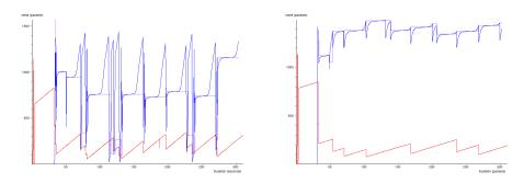
Figure 3: *cwnd* and *last\_max\_cwnd* (purple) histories of Linux 2.6.6+ BicTCP with patch competing against Standard TCP (red). 100Mbit/sec common bottleneck and 162msec RTT experienced by both flows. Bottleneck queuesize is 270 packets. Results shown for Linux 2.6.10 patched (left) and Linux 2.6.10 patched with [DL04] modifications (right).
