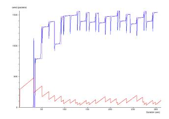
Figure 1: *cwnd* histories of BicTCP version 1.1 (blue) competing against Standard TCP (red). *last\_max\_cwnd* of BicTCP version 1.1 shown in purple with 100Mbit/sec common bottleneck and 162msec RTT experienced by both flows. Bottleneck queuesize is 270 packets. Details of the experimental set-up is given in Appendix A.
