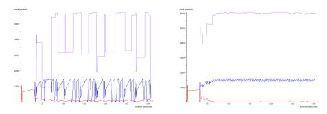
Figure 2: *cwnd* (blue) and *last\_max\_cwnd* (purple) histories of BicTCP Linux 2.6.6+ competing against Standard TCP (red) with 100Mbit/sec common bottleneck and 162msec RTT experienced by both flows. Bottleneck queuesize is 270 packets. Plot on left is Linux 2.6.10 and the plot on the right is Linux 2.6.10 with [DL04] modifications.
